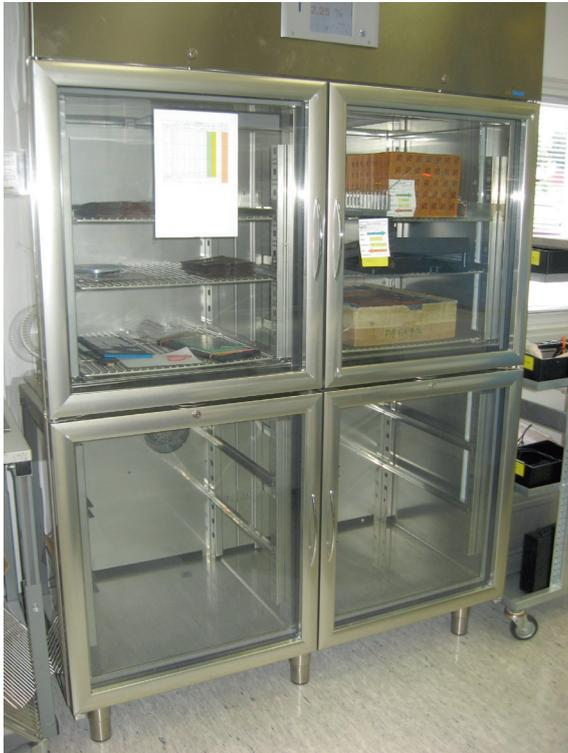
Fig. 2: XSD 1404 dry cabinet (manufactured by Totech)
